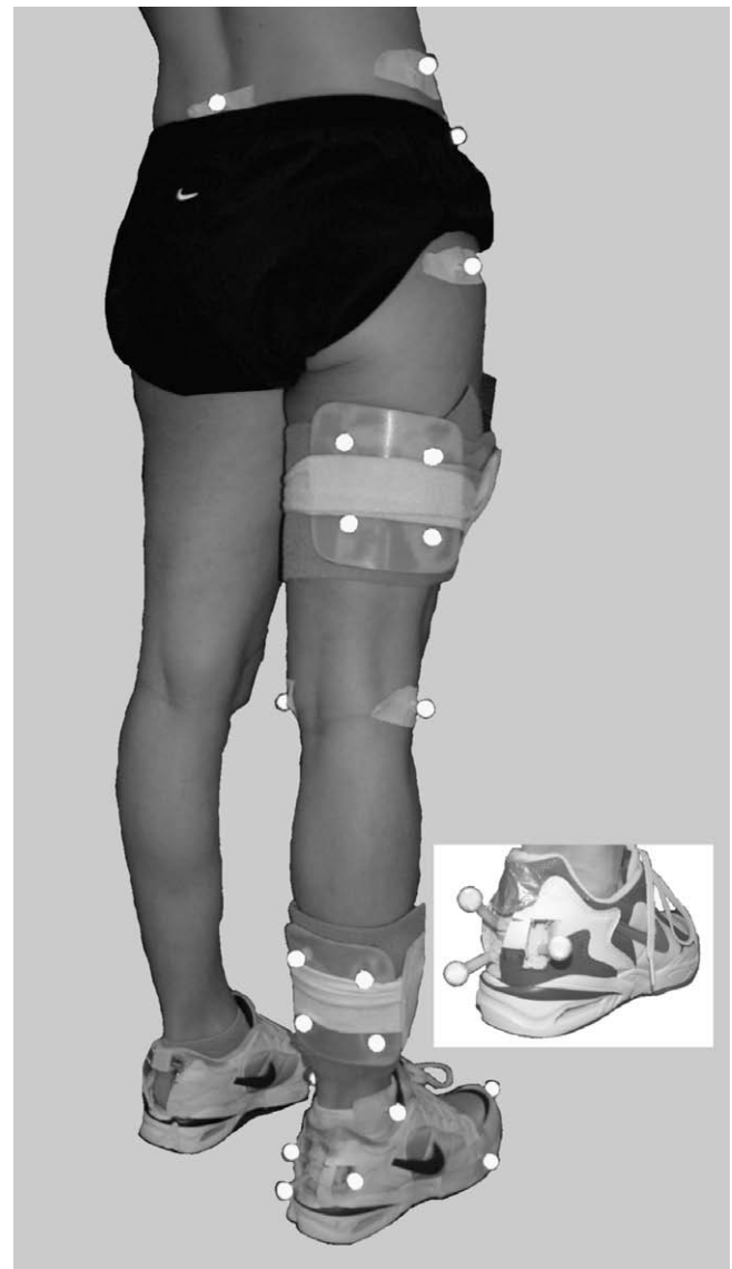
Fig. 2. Retroreflective markers were placed on the pelvis, thigh, shank, and rearfoot. Rearfoot markers were placed directly on the heel through holes in the heel counter of the shoe (inset picture).
